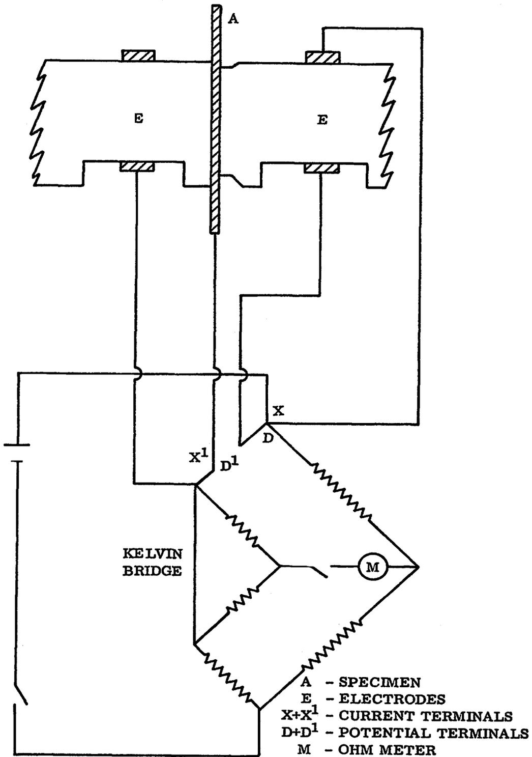
FIGURE 2. Circuit diagram for contact resistance measurements.
